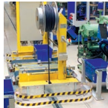
Shuttle car picks full box at injection moulding machine, - simultaneously delivering empty box.
