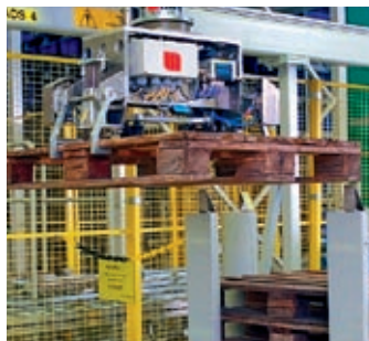
Handling of empty pallets is one of the 4 functions
