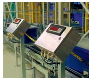
The weight of boxes is double checked - controlling content and number of components
