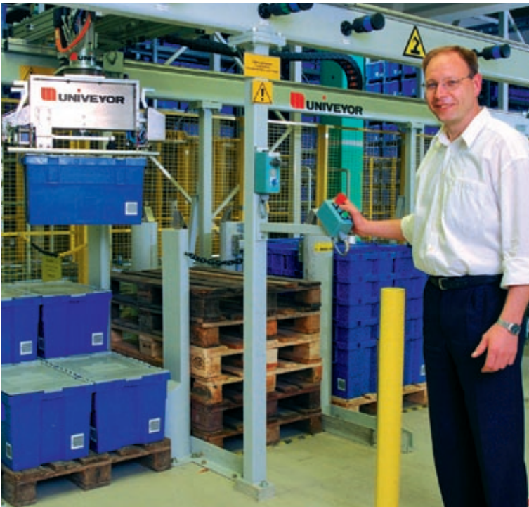
Project manager Leif Hansen, LK. The gantry robot handles boxes, lids and empty pallets.
